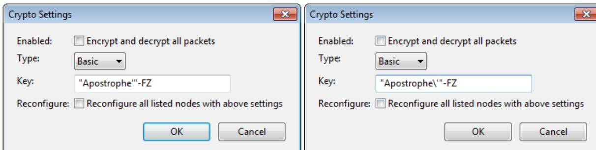
If you check the Reconfigure checkbox, Portal will set all available nodes to use the same encryption settings, using traceroute information to work from the outer edges of your network, in. Refer to the SNAP Reference Manual and SNAP User Guide for more information about encrypted SNAP networks.
