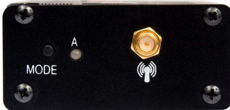
As delivered, LED A glows green when the E10 is powered. Holding the Mode button during startup causes the E10 to bypass the standard SNAP Connect software in the unit. Holding the Mode button for 10 seconds causes the E10 to perform an orderly shutdown.
