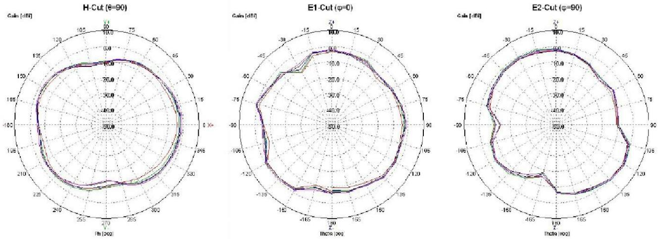
Figure 1.5: ANT-2.4-CW-RAH-RPS Antenna Gains Performance
