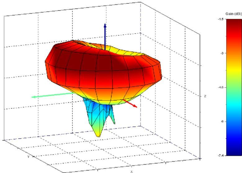
Compact Internal F Antenna Gain Performance at 2370 MHz
