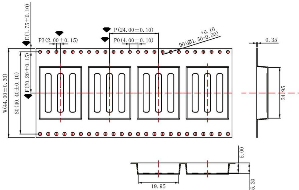
1. Sprocket hole pitch cumulative tolerance: +/-0.2mm.
