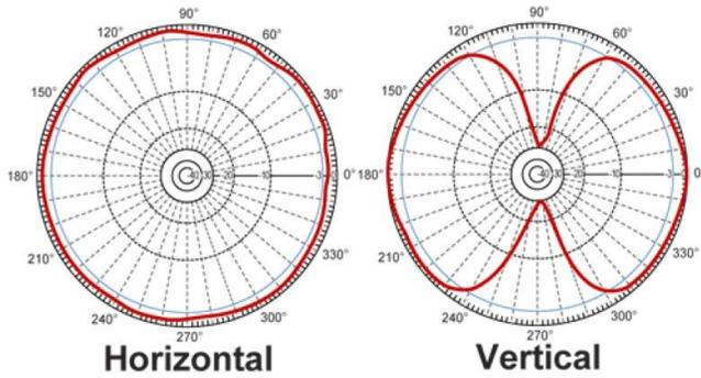
Figure 1.3: HyperLink Technologies HG2405RD-RSP Antenna Gain Performance
