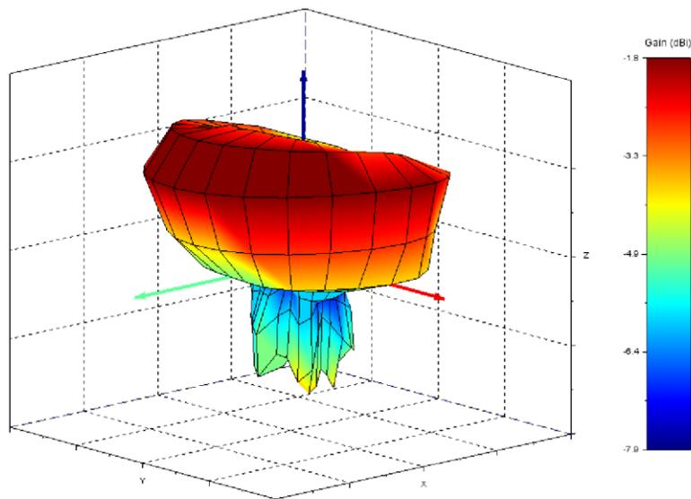
Compact Internal F Antenna Gain Performance at 2440 MHz
