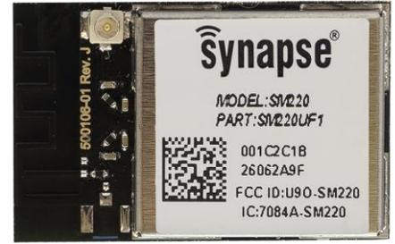
SNAP's on-board Python interpreter provides rapid application development and over-the-air programming, while Atmel's low-power RF single-chip design saves board space and lowers power consumption. The modules provide up to 15 channels of operation in the ISM 2.4GHz frequency band.
